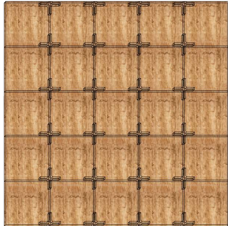
1mx1m Timber Panels
